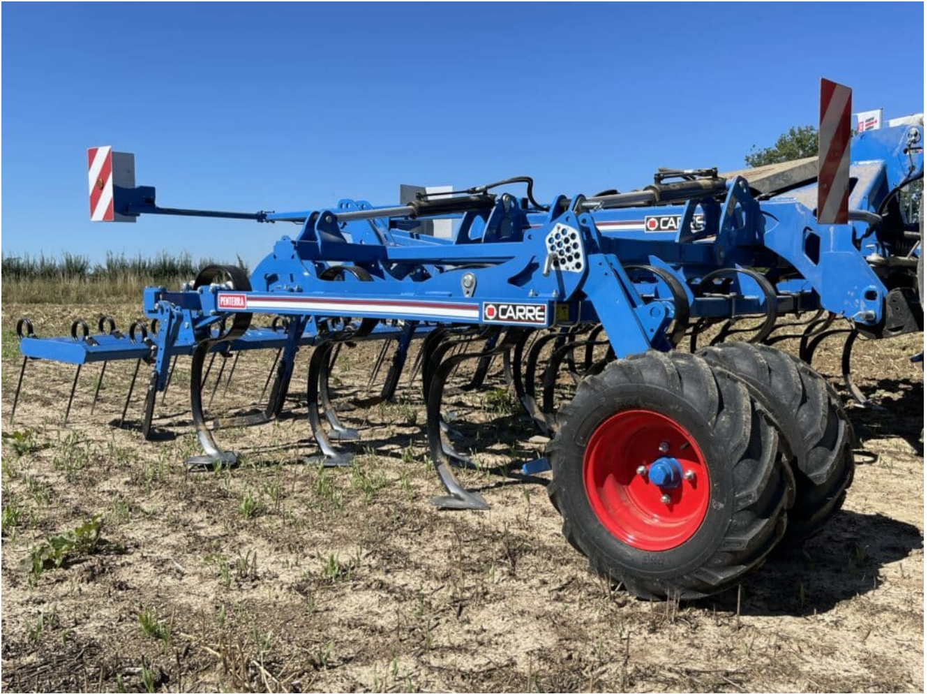
PENTERRA scalping version with 80×12 standard tine + counter spring + reversible share
